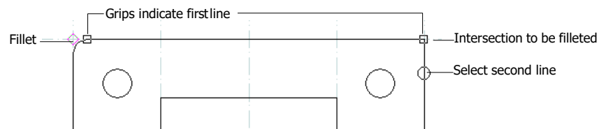
Selecting the first entity for filleting
